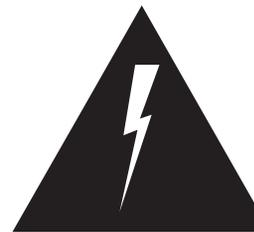
The lightning flash with arrowhead, within an equilateral triangle, is intended to alert the user of the presence of uninsulated "dangerous voltage" within the product's enclosure that may be of sufficient magnitude to constitute a risk of electric shock to persons.
