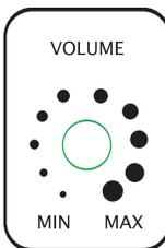
When setting the volume control at the subwoofer, begin with your main speakers playing at a normal listening level and the volume control at the subwoofer completely in the off position (counterclockwise position). Then, begin to turn up the volume at the subwoofer slowly (clockwise) until the desired bass response is achieved. Bass output will then be regulated by your A/V receiver's volume control.
