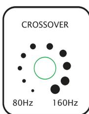
The Crossover Frequency control determines the frequency below which the subwoofer will play. This frequency is manually controlled and is continuously variable between 80-160Hz. You can experiment with which position works best with your main speakers by turning this control until the sound of the low frequency coming from the subwoofer is nicely blended with the sound of your main speakers.
